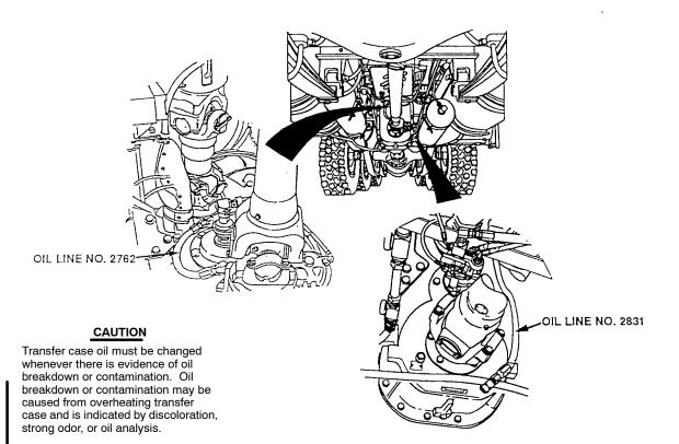
Check transfer case oil lines and fittings for leakage and damage.
