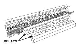
Check wire no. 1590 from HI IDLE SWITCH relay to DDEC HI IDLE relay for loose connections or damage.
