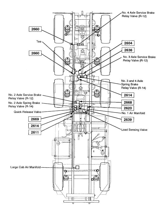
Brake Air Hose Diagram (sheet 2 of 2)
