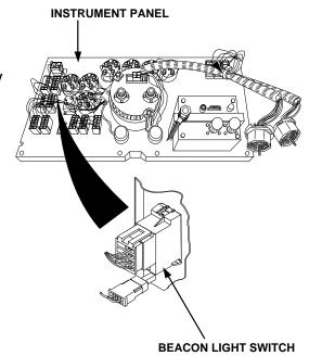
Remove fuse from strobe type beacon light and visually inspect. A fuse will usually "blow" in the center, at the inverted U-shape area. Fuse can also be checked with a multimeter.
