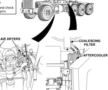
Check aftercooler and coalescing filter for air leaks.
