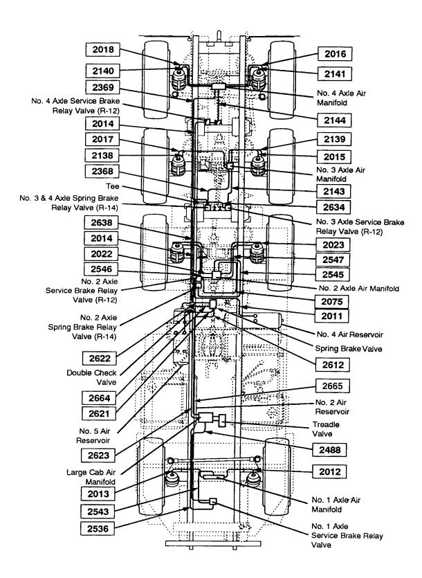
Brake Air Hose Diagram (sheet 1 of 2)
