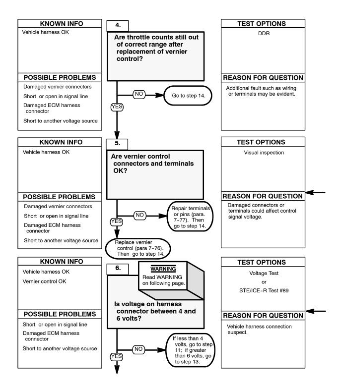
Inspect terminals at vernier control connector (sensor side and harness side) for damage; bent, corroded, and unseated pins or sockets
