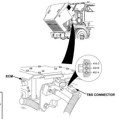
Inspect terminals at TBS connectors (sensor side and harness side) for damage; bent, corroded, and unseated pins or sockets.
