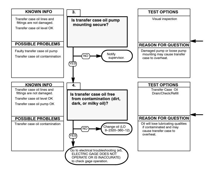
Check transfer case oil pump for damage, and for loose or missing mounting hardware.
