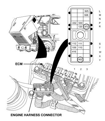
Check terminals at ECM engine harness connector (both ECM and harness side) for damage; bent, corroded, and unseated pins or sockets.
