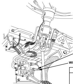
Check ground wire no. 1435 from low air pressure switches for loose connections or damage.
