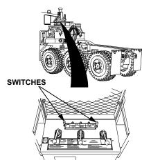
Check wire no. 1154A from left ENGINE SPEED CONTROL switch to HI IDLE SWITCH relay for loose connections, damage, and continuity test.
