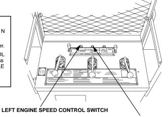
**PUSH TO LOCK ENGINE @ HIGH IDLE SWITCH**
