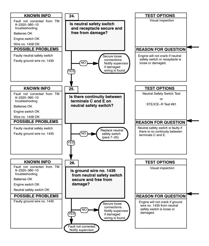
Check neutral safety switch and receptacle for loose connections or damage.
