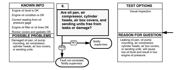
Check oil pan, air compressor, cylinder heads, air box covers, and sending units for leakage or damage.
