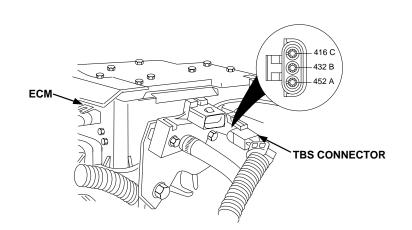
Check terminals at ECM engine harness connector (both ECM and harness side) for damage; bent, corroded,and unseated pins or sockets.
