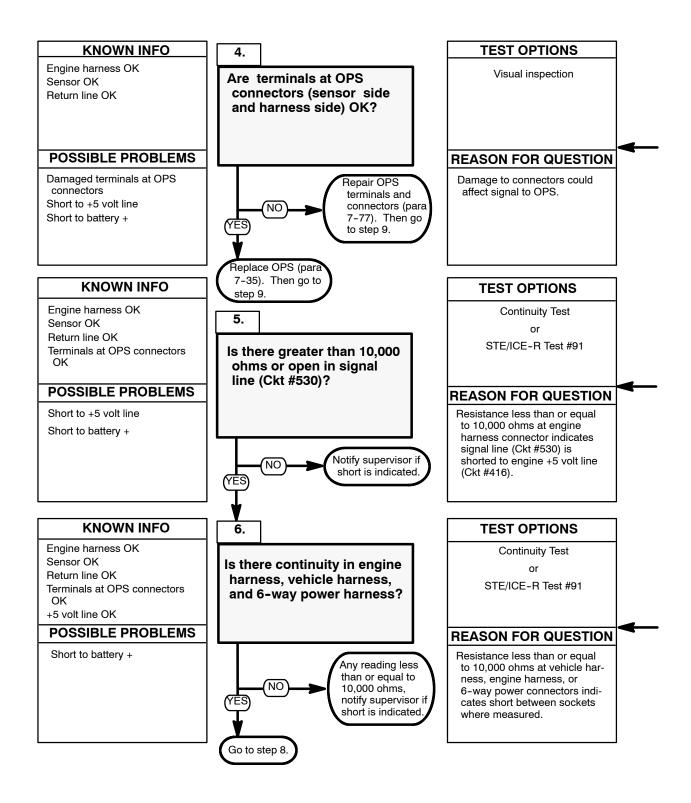
Inspect terminals at OPS connectors (sensor side and harness side) form damage; bent, corroded, and unseated pins or sockets.
