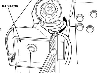
**COOLANT LEVEL SENSOR PROBE**
