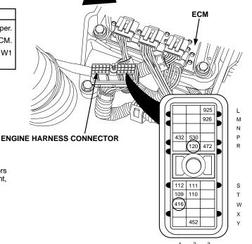
Inspect OTS and terminals at OTS connectors (both sensor and harness sides) for damage; bent, corroded, and unseated pins or sockets
