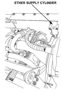
Check ether line between supply cylinder and engine for leaks and damage.
