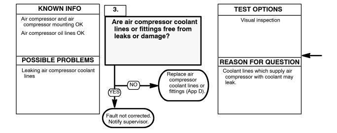
Check air compressor coolant lines and fittings for leakage and damage.
