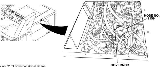
Check no. 2159 governor signal air line and fittings at governor and no. 1 air tank for air leakage and damage.
