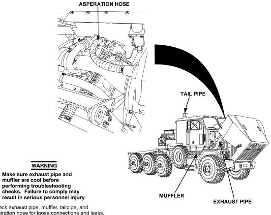
Check exhaust pipe, muffler, tailpipe, and aspiration hose for loose connections and leaks.
