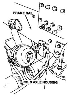
Measure distance from top of no. 3 axle housing to bottom of frame rail on left and right sides. Distance should be 9 in (22.9 cm) on both sides.
