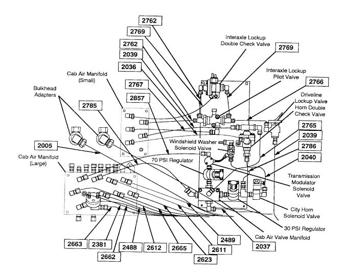
Top View of Cab Air Valve Assembly and Manifold
