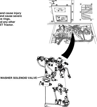
Check ground wire no. 1435 from washer control valve for loose connections or damage.
