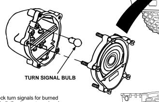
Check turn signals for burned out bulb if only one turn signal does not operate.
