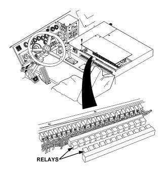
Check wire no. 1154 from P.T.O. HI IDLE relay to ENGINE SPEED CONTROL switches for loose connections, damage, and continuity test.
