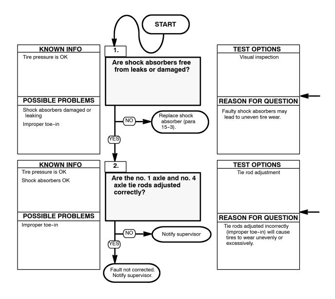
Inspect tires for excessive wear. Tires that have flat spots indicate a defective shock absorber. Inspect shock absorbers for leaks or damage.
