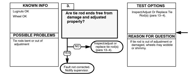
Check front and rear tie rods for cracks, bends, and/or loose or damaged mounting hardware. Refer to para 13-4 for tie rod adjustment and/or replacement procedures.
