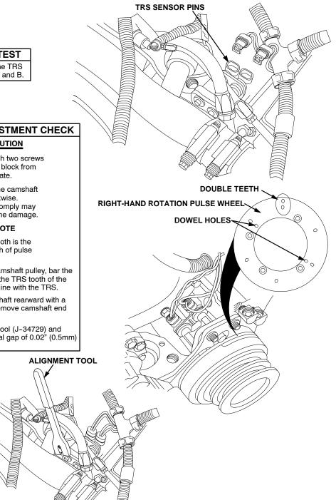
Read resistance of the TRS across sensor pins A and B.
