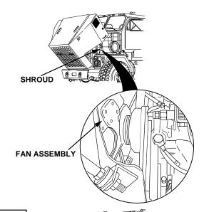
Check fan assembly and shroud for damage.
