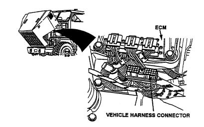
Check terminals at both vehicle harness and 6-way power harness connectors (both the ECM and harness side) for damage; bent, corroded and unseated pins or sockets.
