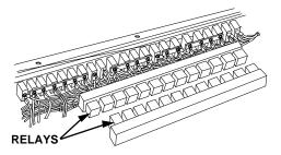
Check wire no. 1154B from right ENGINE SPEED CONTROL switch to HI IDLE SWITCH relay for loose connections, damage, and continuity.
