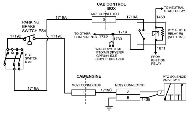
**PTO WIRING DIAGRAM**
