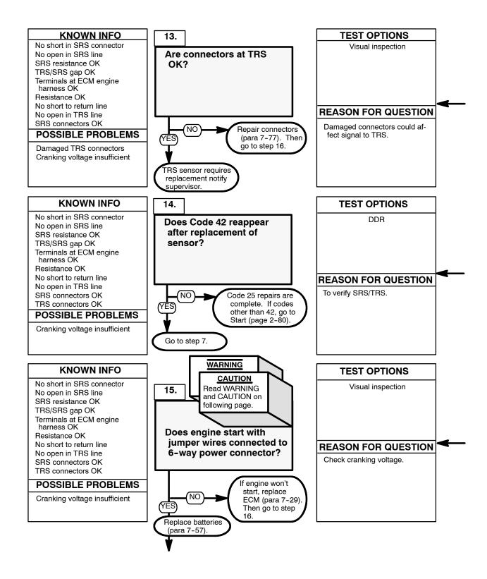
Check connectors at TRS (both harness side and SRS side) for damage; bent, corroded, and unseated pins or sockets, or bad contacts.
