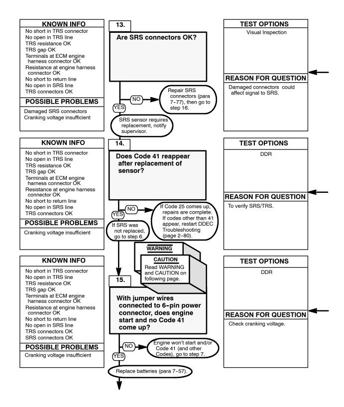
Check connectors at SRS (both harness side and SRS side) for damage; bent, corroded, and unseated pins or sockets, or bad contacts.
