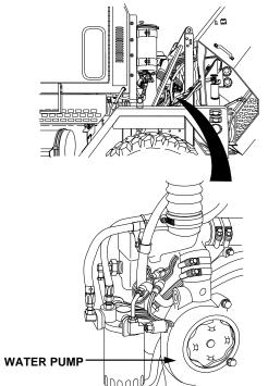
Check water pump for leaks or damage.
