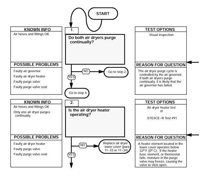
Check purge valve on both air dryers for air leakage.
