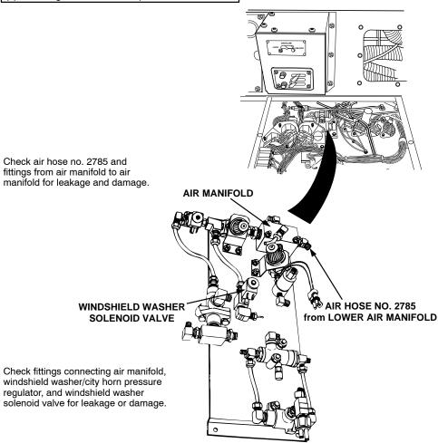
Check air hose no. 2785 and fittings from air manifold to air manifold for leakage and damage.
