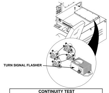
Check ground wire no. 1435 from turn signal flasher for loose connections or damage.
