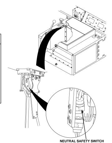
Check ground wire no. 1435 from neutral safety switch to ground for loose connections and damage.
