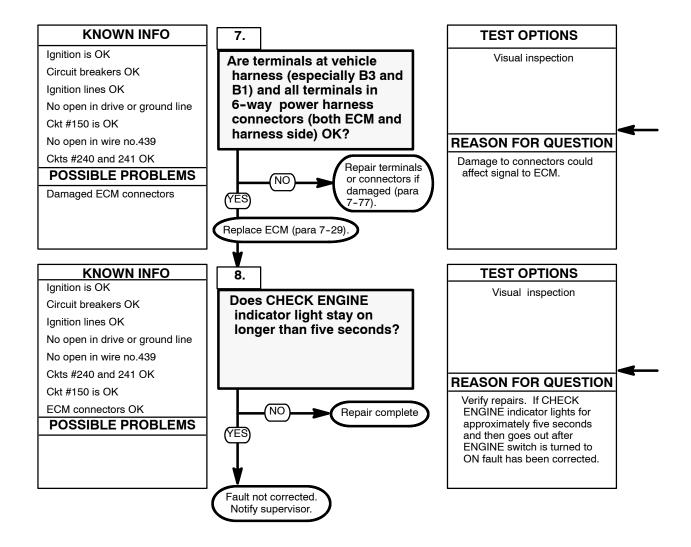
Check terminals at vehicle harness (especially B3 and B1) and all the terminals in 6-way power harness connectors (both the ECM and harness side) for damage; bent, corroded and unseated pins or sockets.
