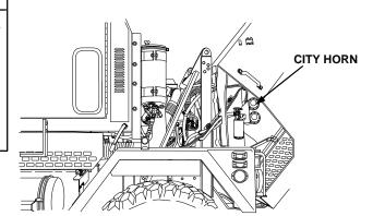
Check air line no. 2036 at city air horn for leakage and restrictions.
