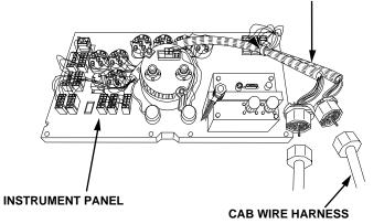
Remove instrument panel (para 7-13) and check if cab wire harness is connected securely to instrument panel wire harness.
