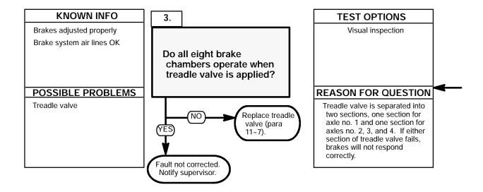
Apply service brake while assistant observes the eight brake chambers for movement of rod.
