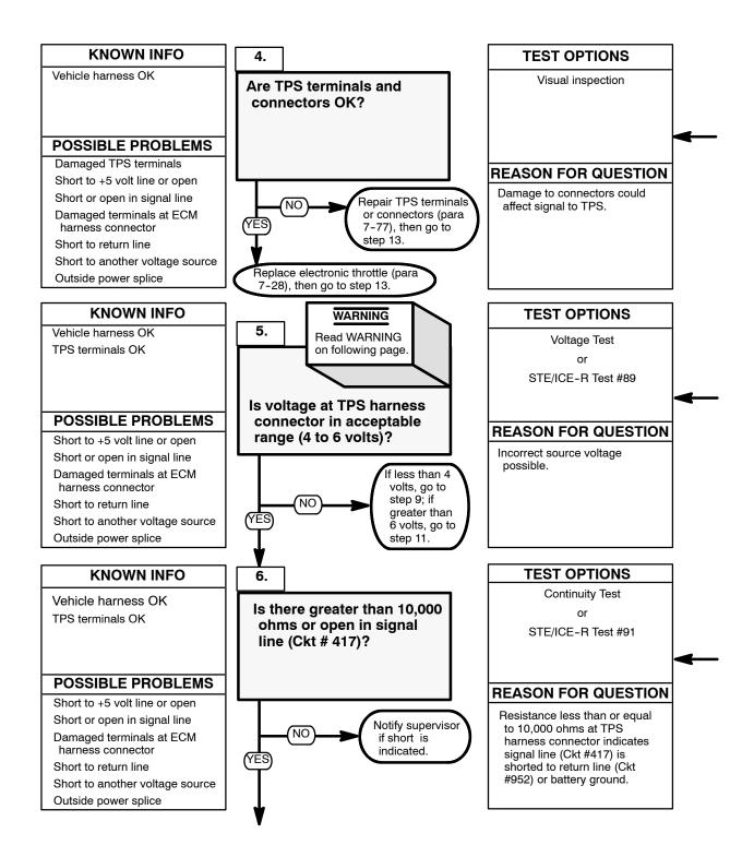
Inspect TPS and terminals at TPS connectors (sensor side and harness side) for damage; bent, corroded, and unseated pins or sockets.
