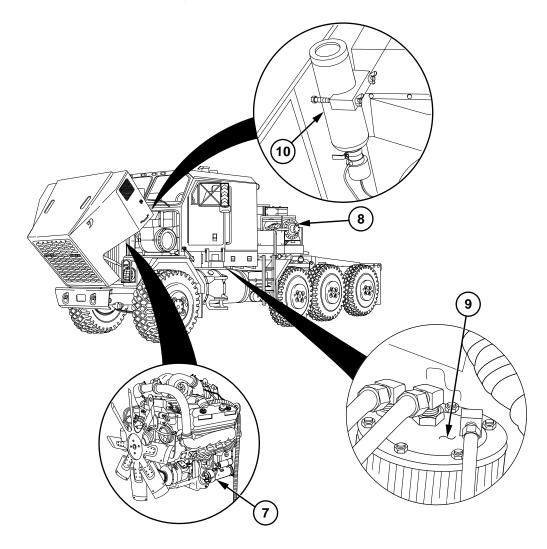
The starter motor solenoid receives 24 Vdc from the storage batteries through the engine starter magnetic switch auxiliary contacts and the neutral start relay. If the transmission range selector is not in the N (neutral) position prior to startup, the engine cannot be started.
