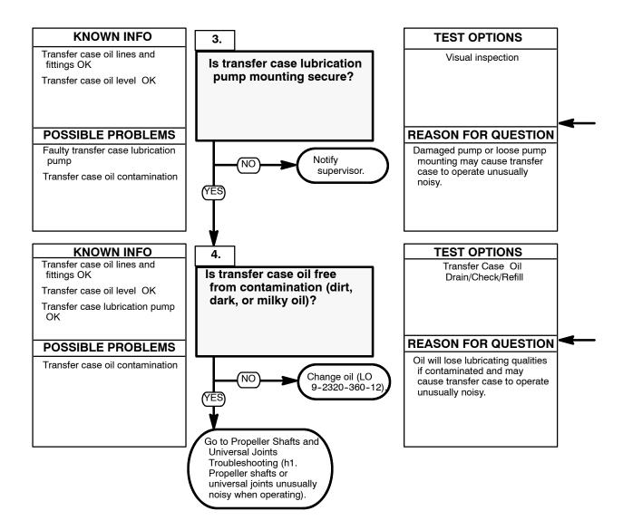
Check transfer case lubrication pump for damage, and for loose or missing mounting hardware.
