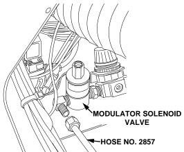
Inspect air line no. 2857 in doghouse, at manifold block and outside cab for leaks, kinks, or damage.
