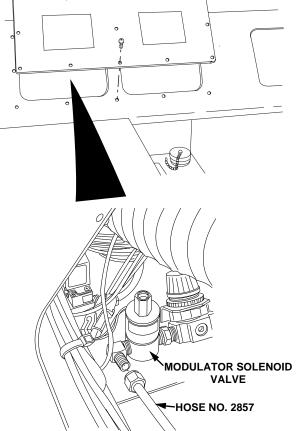
Inspect air line no. 2857 in doghouse, at manifold block and outside cab for leaks, kinks, or damage.
