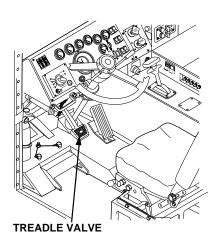
Press and hold treadle valve while assistant checks brake chambers for air leaks.
